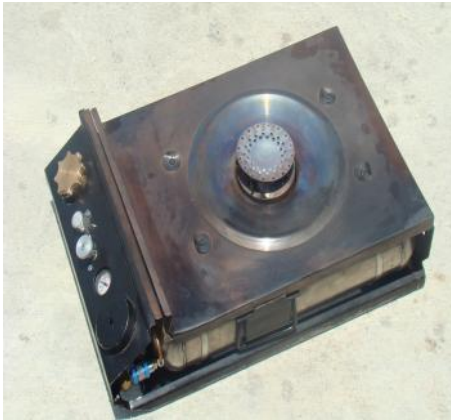
Multi Fuel Burner
