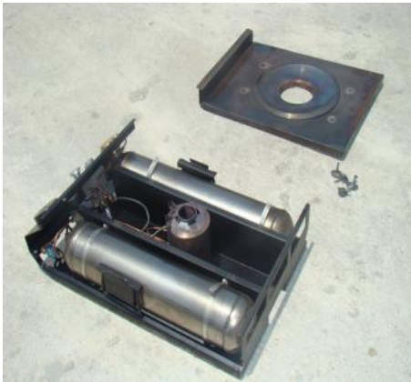
Multi Fuel Burner - Top Cover Removed
